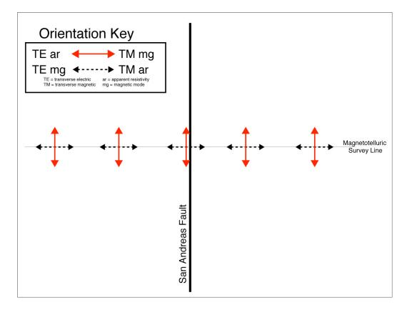
Fault parallel apparent resistivity is shown in the TE images, and fault perpendicular apparent resistivity is shown in the TM images. In general, the seminar participants agreed that there was a low resistivity feature under the Middle Mountain region.
